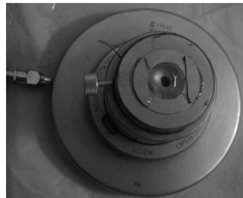
Figure 1 – The artificial anterior chamber used for the experiment
