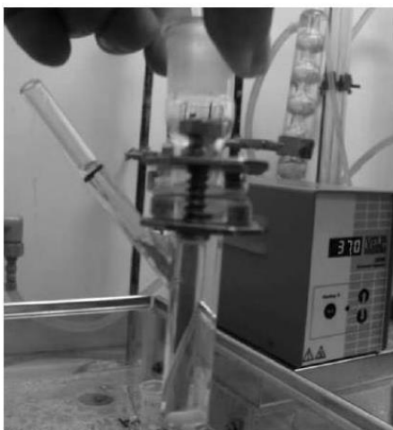
Figure 6 – The Franz-cell used for experimentation.
